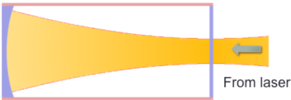
Figure 55: Schematic ideal profile of beam within cavity
