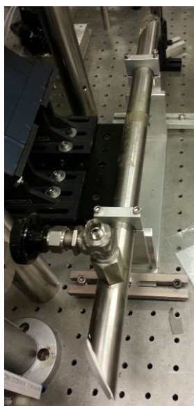
Figure 19: Image of ^{14}\text{NO} reference cell. There is a separate cell filled with ^{15}\text{NO}
