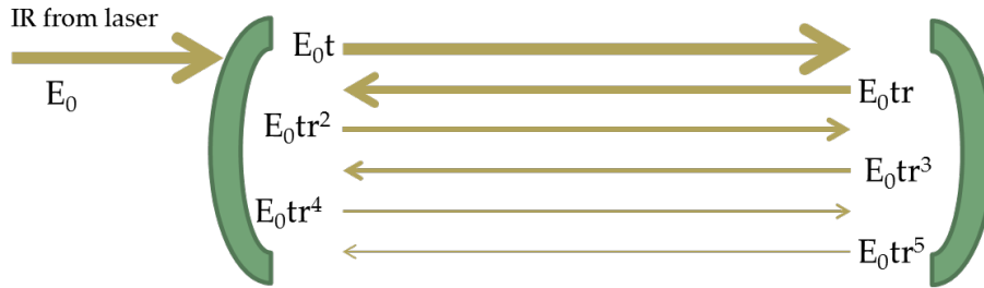
Figure 2: Constructive interference of the electric field of light in a resonant cavity
