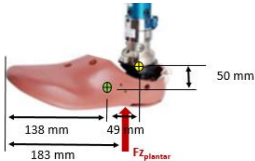
Figure 7.49. Estimated location of the center of mass, center of pressure, and center of ankle rotation location for the Mil-Lx.
